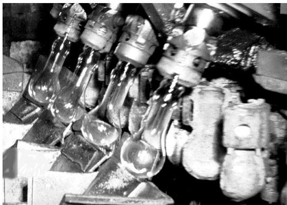
Production of lamp bulbs on a carrousel machine. The molds are rotating to prevent mold seams. A similar technology is used to produce wine glasses.
